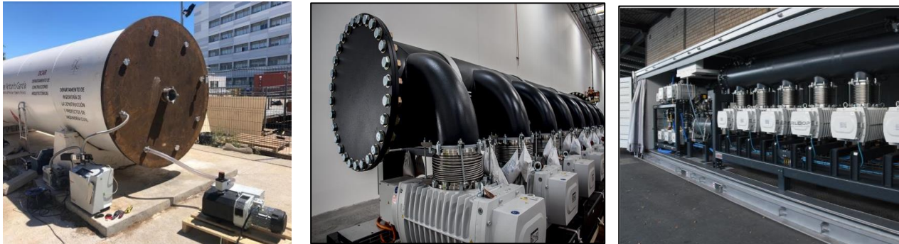
Figure 2. Tube and pressure maintenance system test (left side) at Universitat Politècnica de València, Spain (Hyperloop UPV, 2019). Vacuum pumps (middle) to be tested in Virgin Hyperloop One (Virgin Hyperloop One, 2016b). A vacuum pump unit (right side) with a modular housing to be tested in HyperloopTT (HyperloopTT, 2019)
