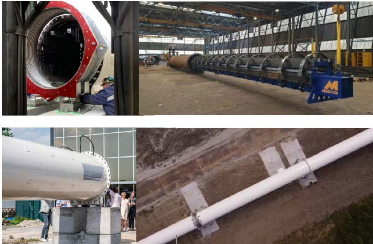
Figure 54. Manufacturing tube process (above). Source: Mercon. Infrastructure prototype at the EHC site in Groningen (below). Source: HARDT
