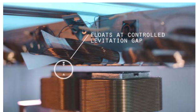
Figure 70. Sketch of EMS with permanent magnet in the centre of steel core and close to the magnets at HARDT's propulsion and levitation demo
