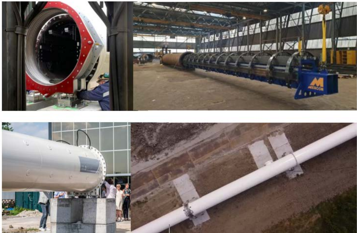
Figure 57. Manufacturing tube process (above). Source: Mercon. Infrastructure prototype at the EHC site in Groningen (below). Source: HARDT
