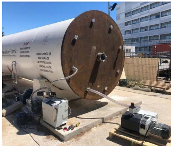
Figure 63. Vacuum system for testing purposes. Source: Universidad Politécnica de Valencia
