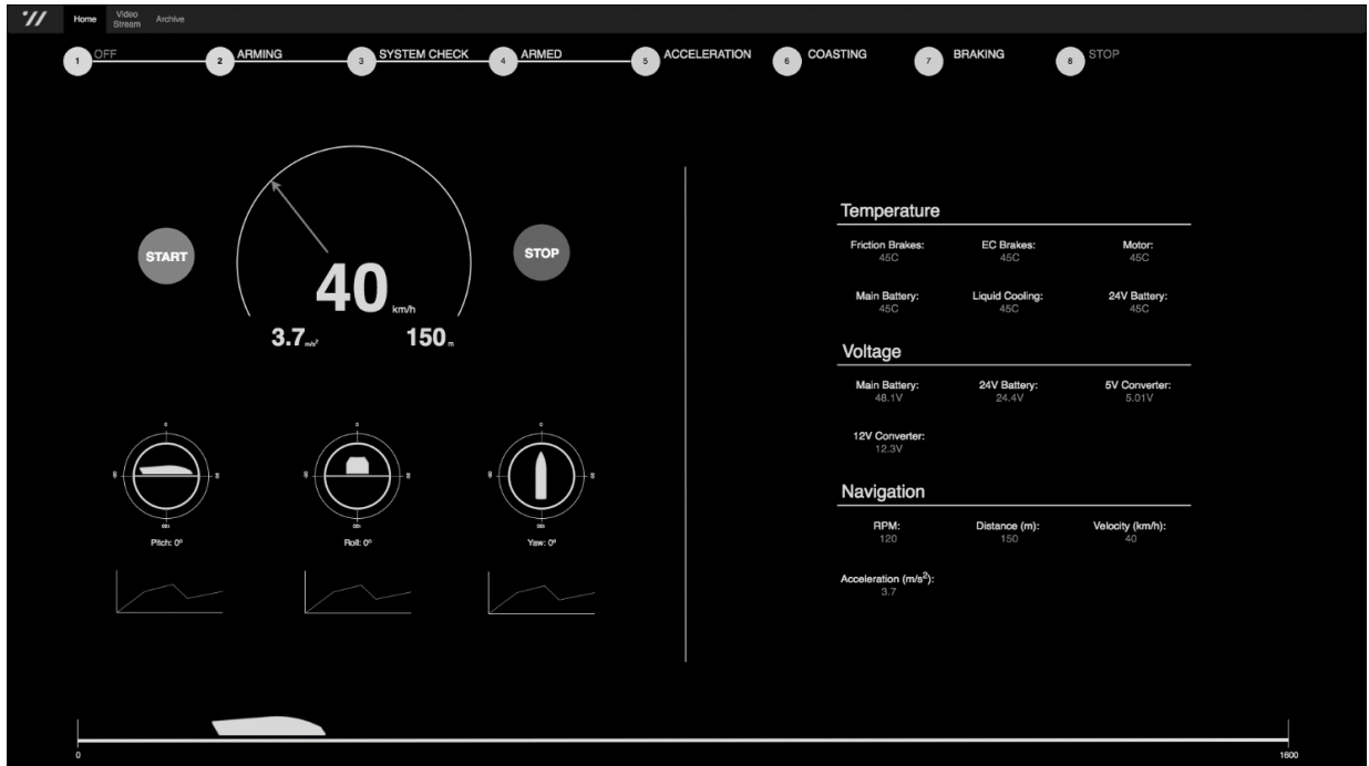
Fig. 10.: UI with minimal required control elements and real-time data visualization components
